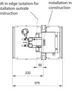
Built in edge signifies depth of damper insertion into wall
