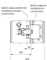
Built in edge signifies depth of damper insertion into wall
